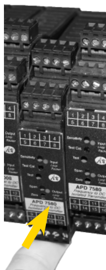
Tilt module downward slightly and clip Lower Mount to bottom edge of 35 mm DIN rail.
