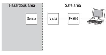
Fig. 7. Configuring the SINEAX V 624, types 624-33/34/93/94 when the sensor is in the hazardous area. For this case the switch on the interface of the PK 610 must be set to "ON" or "OFF", see Fig. 6.
