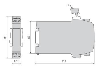
Fig. 12. SINEAX V 624 in housing **P12/17 St** clipped onto a rail «G» (35 × 15 mm or  $35 \times 7.5$  mm, acc. to EN 50 022), screw terminals pluggable.
