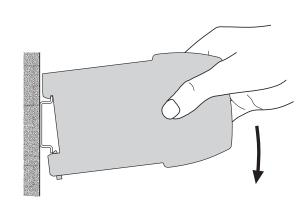
Fig. 3. Mounting onto top-hat rails  $35 \times 15$  or  $35 \times 7.5$  mm.
