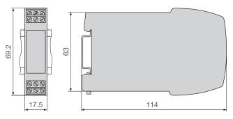
Fig. 11. SINEAX V 624 in housing P12/17 clipped onto a top-hat rail (35  $\times$  15 mm or  $35 \times 7.5$  mm, acc. to EN 50 022), screw terminals not pluggable.
