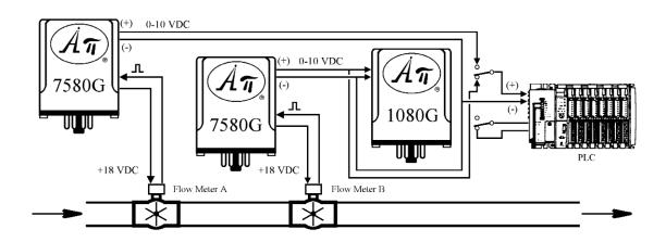
The second set of relay contacts of the **API 1080 G** provides a PLC binary input with a closure to indicate which flow meter is selected.
