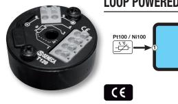
T120 is a converter for Thermoresistance PT100/Ni100 with 2,3,4 wires and convert it into 4..20mA loop powered signal. It's completely configurable through PC software. T120 is suitable for in-head mounting (Pt100). The output signal is not isolated from the input one.
